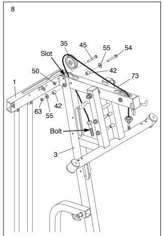
Feed the bolt on the High Cable (73) under the wlded tube on the Press Frame (12) as shown. Wrap the High Cable around a 4" Pulley (35) in the direction shown. Attach the Pulley to the Press Frame (12) with a 3/8" x 8 1/2" Bolt (59) and a 3/8" Nylon Locknut (50).
